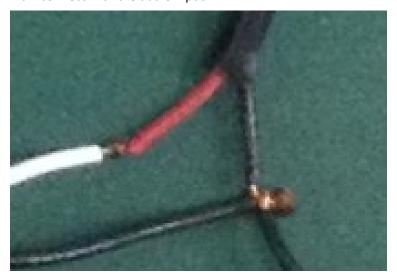
The white cable is the positive pole, the black cable is the negative pole
