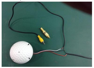
(the functions of the yellow connector and the golden connector are same ) pic1:connect with the power
