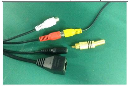
3. Connect the audio AV port to the audio input connector of the camera(red one), the connection is finished.
